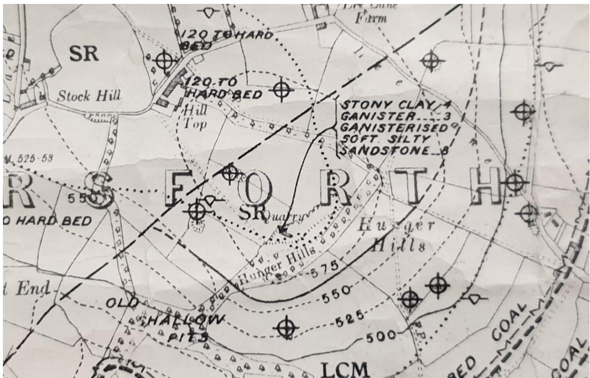
Figure 5: Detail of quarry and bell mines Hunger Hills c.1840? Bell mines are circles with crosses.
